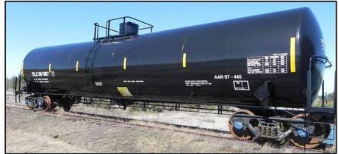
DOT/TC-117J100W Tank Car for Flammable Liquid Service
