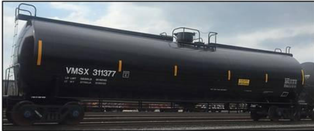
DOT/TC-117R100W Tank Car for Flammable Liquid Service
